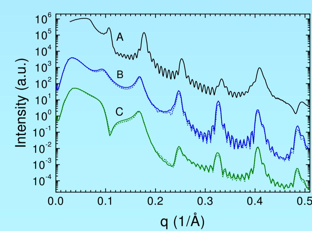
Soft x-ray resonant magnetic scattering (BESSY II, Berlin) – **ALICE diffractometer** - reflectivity curves with circularly polarized x-rays tuned to L<sub>3</sub> Co (778 eV) and L<sub>3</sub> Ni (853 eV) absorption edges.
