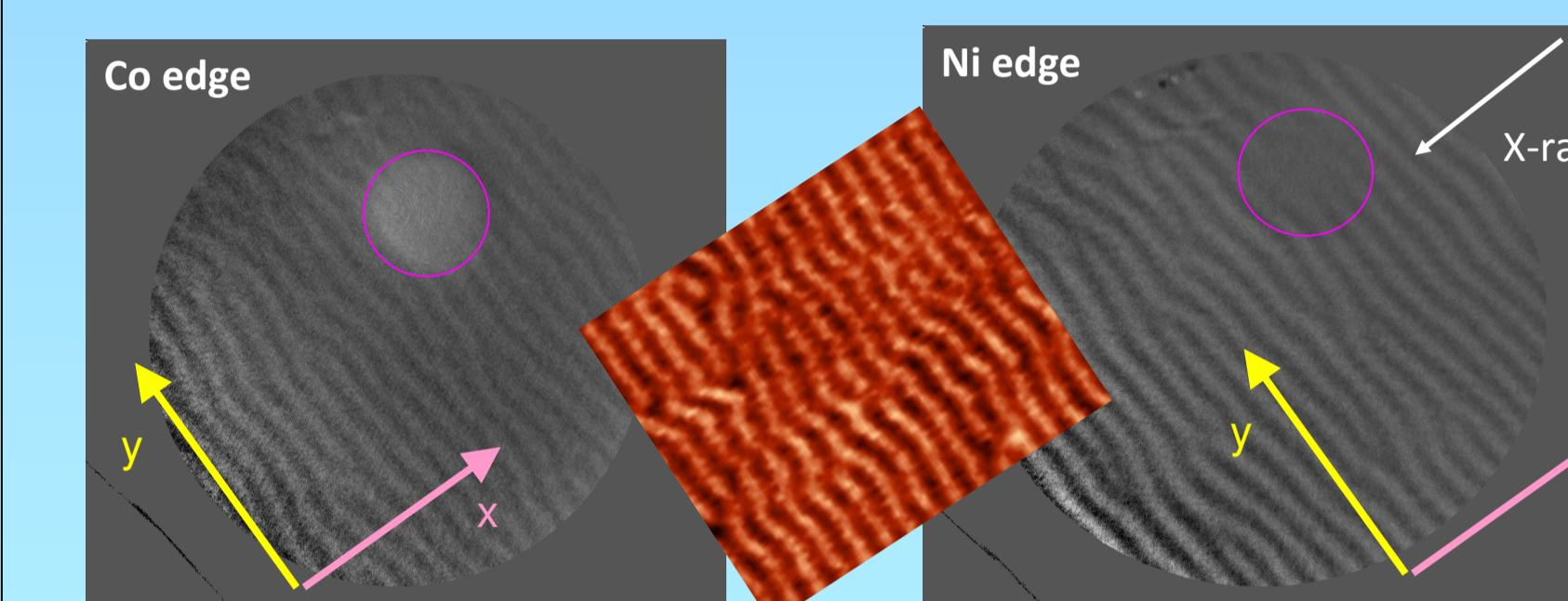
Sample was initially saturated in-plane by magnetic field applied along y axis. Stripe domains oriented along x,y' axis were produced. Images size 5x5μm.
