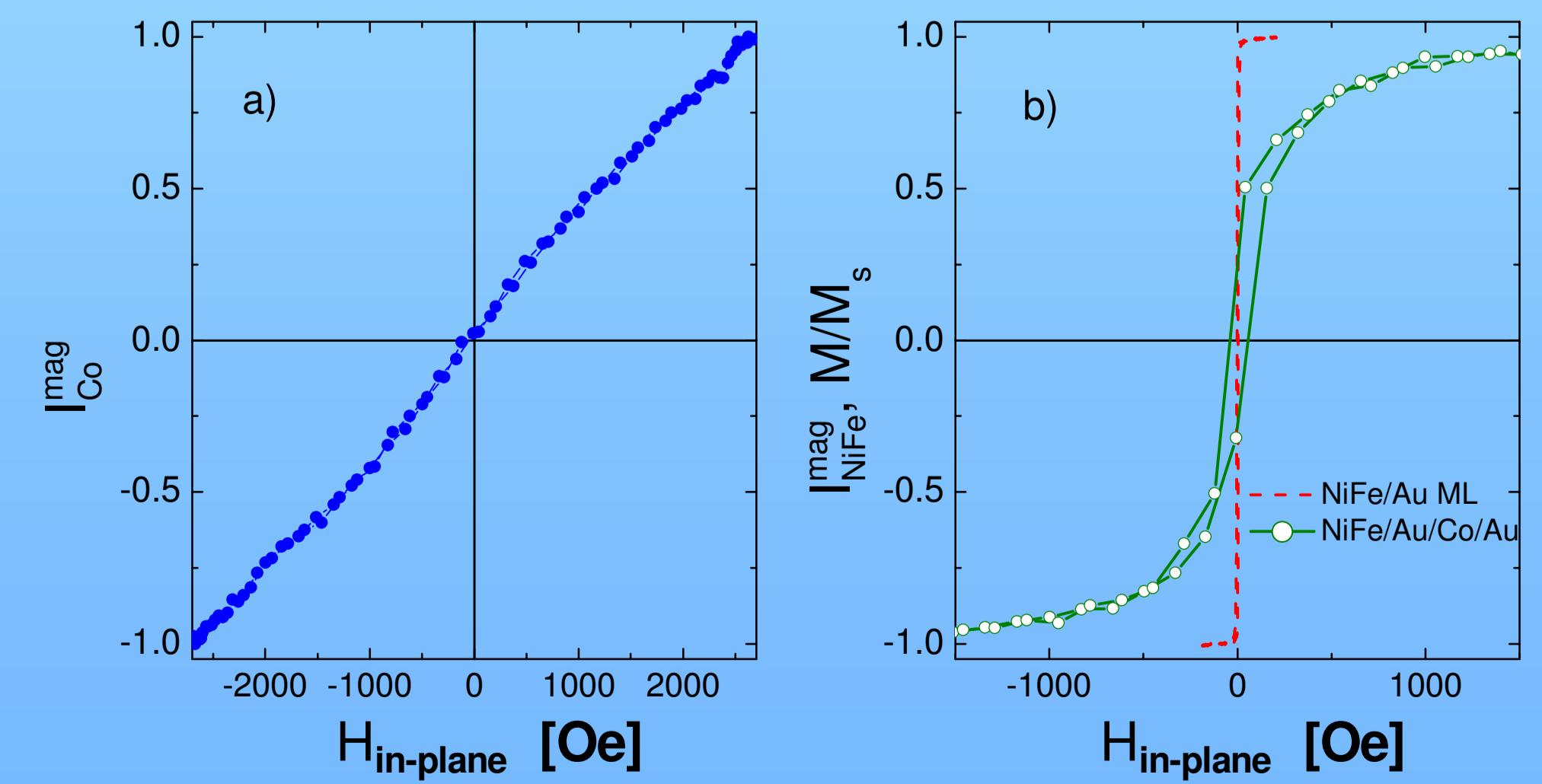
Normalized magnetic signals versus H determined from curves measured at L<sub>3</sub> Co and L<sub>3</sub> Ni and incident angle of 8.5°
