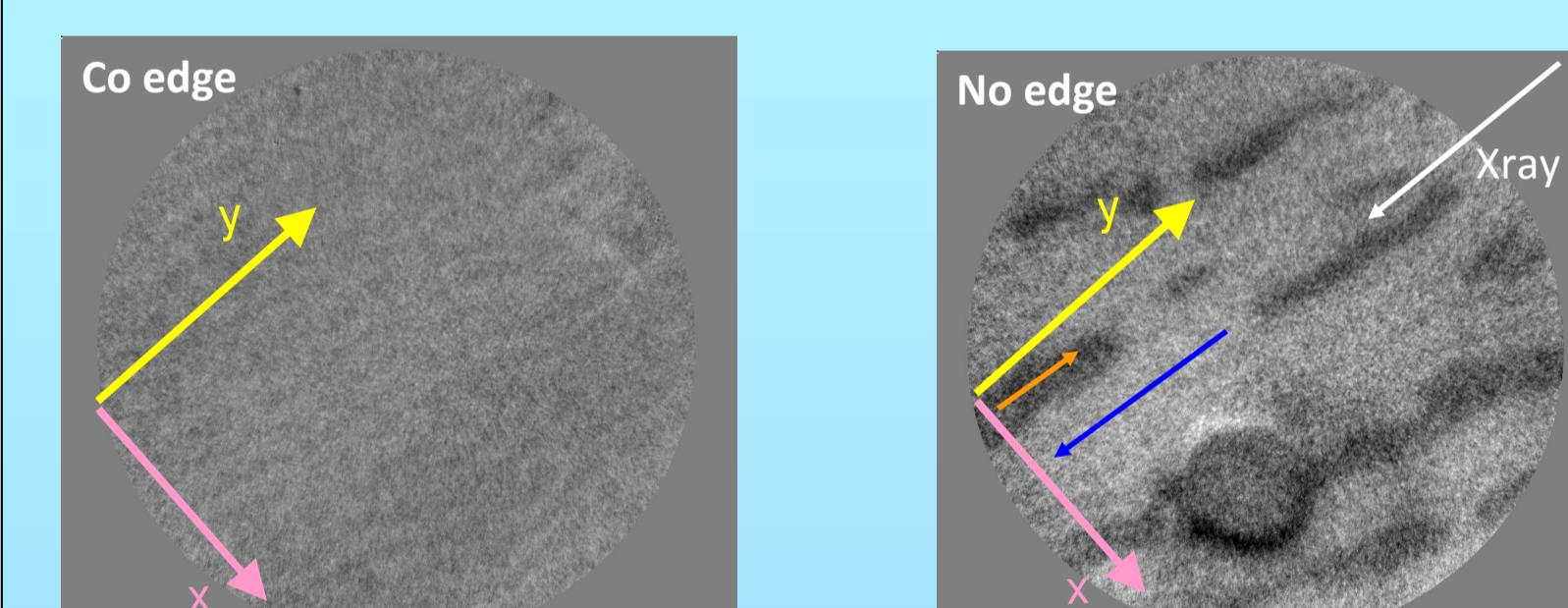
There is weak contrast related to stripe domains (in both Co and NiFe). Additionally **macrodomains**, with large contrast, are visible in NiFe layers (this contrast could be related to y magnetization component).
