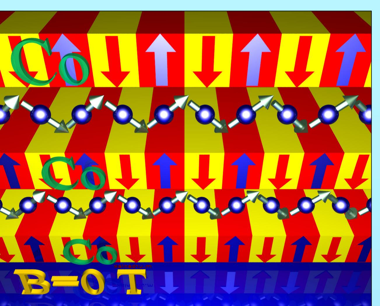
This MLs display the **giant magnetoresistance (GMR)**:
