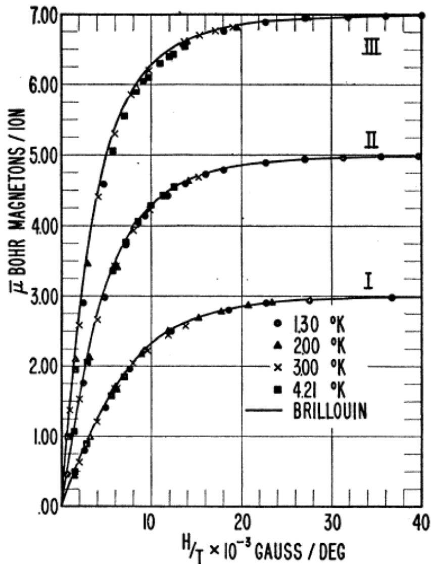
FIG. 3. Plot of average magnetic moment per ion,  $\bar{\mu}$  vs  $H/T$  for (I) potassium chromium alum ( $J=S=3/2$ ), (II) iron ammonium alum ( $J=S=5/2$ ), and (III) gadolinium sulfate octahydrate ( $J=S=7/2$ ).  $g=2$  in all cases, the normalizing point is at the highest value of  $H/T$ .
