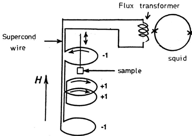
Fig.3 Diagram of SQUID magnetometer
