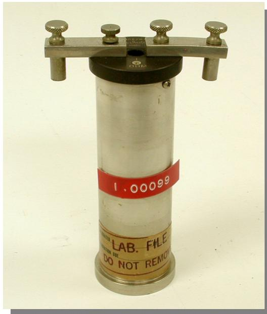
The standard is equipped with large contacts to minimize effects of the contact resistance
