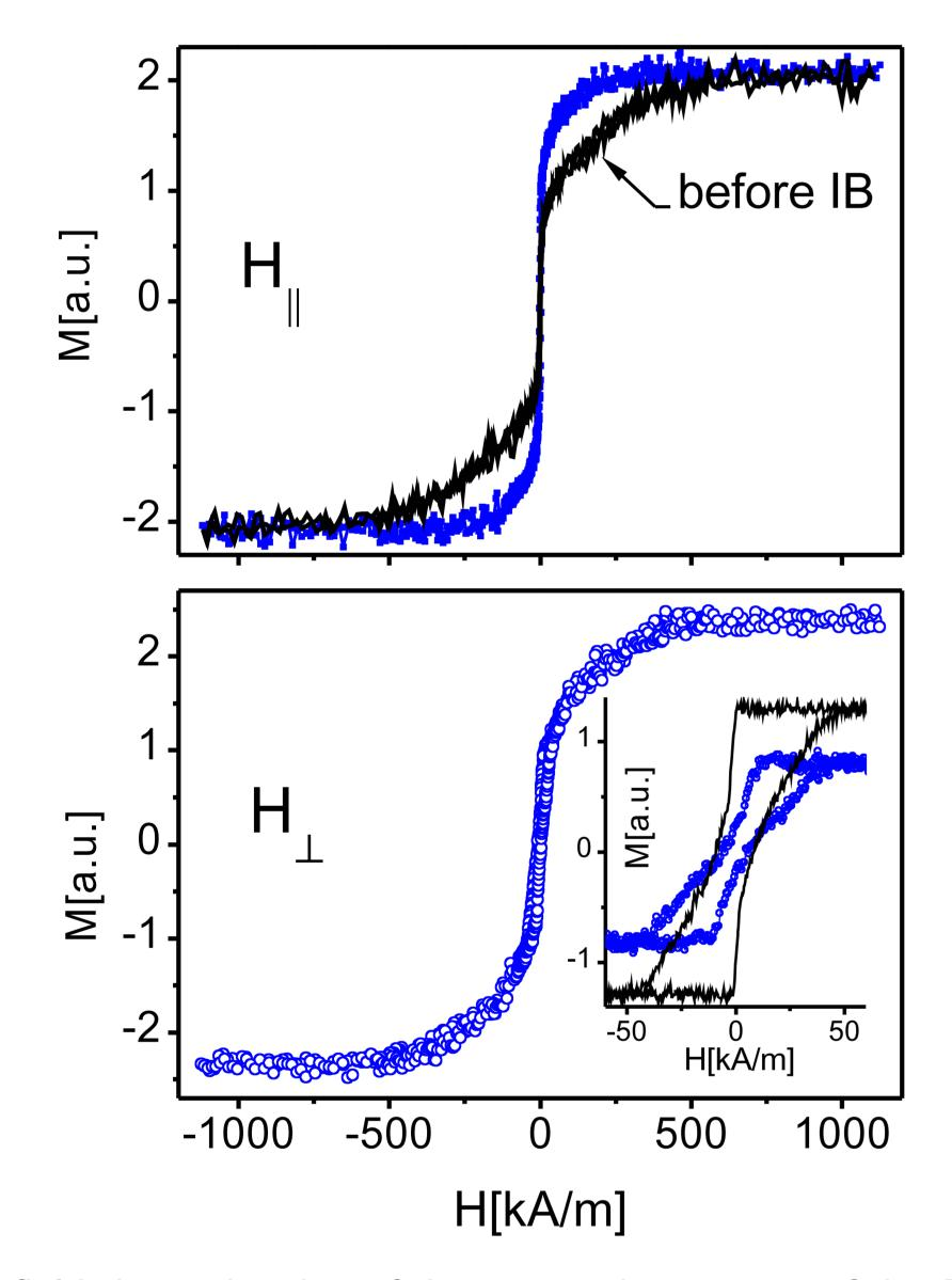
The field dependencies of the magnetic moment of the  $[\text{Co}_1(0.6\text{nm})/\text{Au}(4\text{nm})/\text{Co}_2(1\text{nm})/\text{Au}(4\text{nm})]_4$  ML before and after the IB with He<sup>+</sup> (10keV,  $6\text{x}10^{14}\text{ions cm}^{-2}$ ). The upper panel shows the dependencies measured with the field applied in the sample plane and the lower for the perpendicular configuration. The inset shows the small field range hysteresis of the Co layers.
