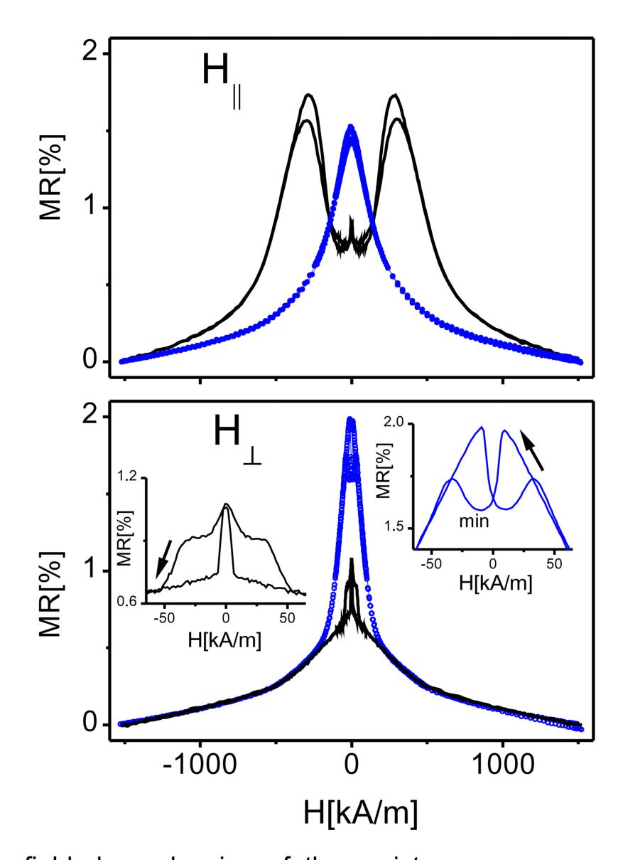
The field dependencies of the resistance corresponding to M(H) dependencies shown left. The upper panel shows the dependencies measured with the field applied in-plane and the lower for the perpendicular configuration. The insets show the expanded view of the small field range resistance changes. The arrows show a field sweep direction.
