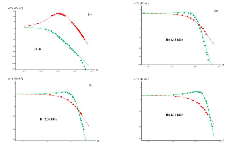
Fig1. Ultrasonic attenuation in MnP. The dashed lines correspond to  $T < T_C$  and the continuous lines to  $T > T_C$ . The data are taken from Ref. [4].
