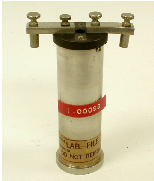
Honeywell four-terminal 1 Ohm resistance standard
