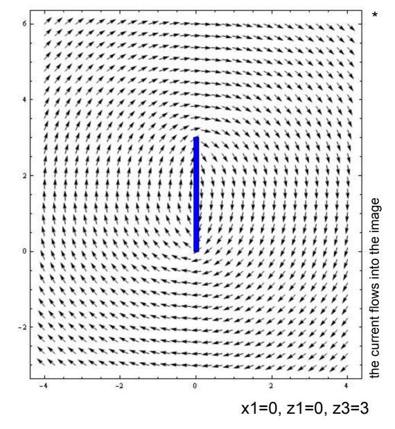
\*for better viewing the plot shows only the direction of the field (vectors' length is constant)
