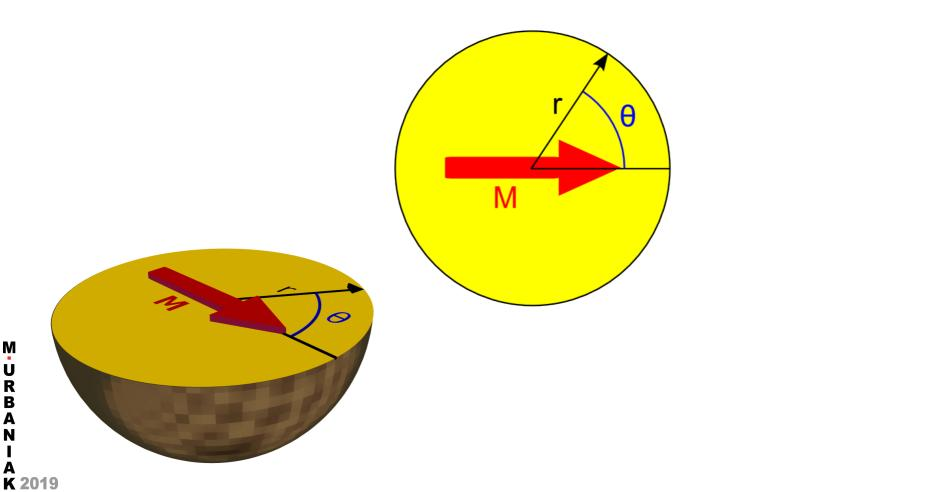
We assume that the sphere is homogeneously magnetized in *z* direction and copying from Bartelmann [7] and Hauser [3] we seek the magnetic potential. We have:  $\vec{z}_{i}$
