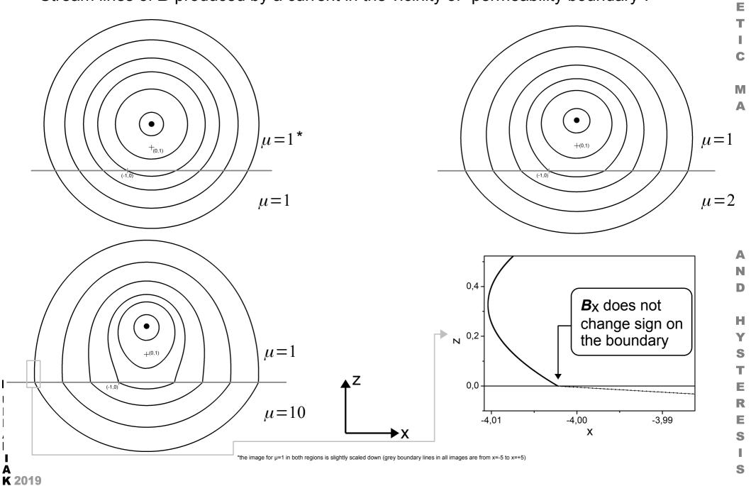
•Stream lines of **B** produced by a current in the vicinity of "permeability boundary":
