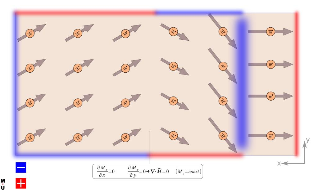
• Change of the direction or the magnitude of the magnetization is not necessarily accompanied by the presence of magnetic charges
