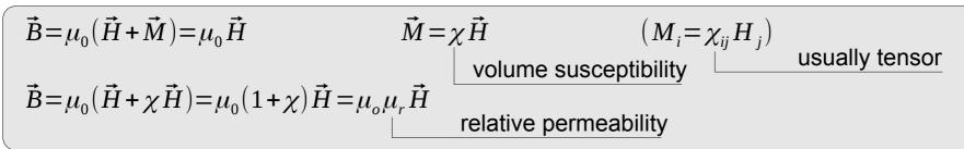
The sphere of permeability  $\mu$  is placed in an external field **B**<sub>0</sub> [1,8]. The magnetization of the sphere depends now on the field strength. From previous page we have:
