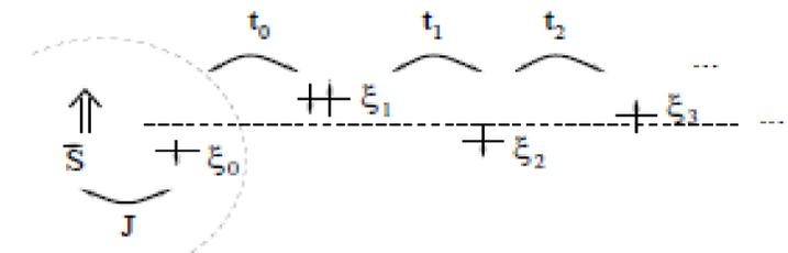
Fig. Scheme of log. discretized metallic band and Wilson chain with exponentially decaying hopping
