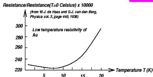
Fig. Electrical resistivity of Au metal with impurities
