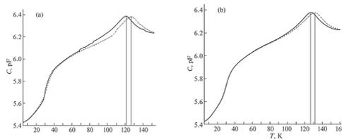
**Fig. 1. Temperature dependences of capacitance  $C$  measured for Fe<sub>20</sub>MAP + KDP nanocomposite on cooling (dotted line) and heating (solid line) in (a) zero field and (b) external field of  $B = 10$  T. Vertical lines indicate the positions of maximum on the  $C(T)$  curves.**
