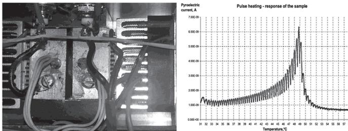
**Fig. 1. Sample holder for dynamic measurements (A), pyroelectric response of TGS sample on pulse temperature waveform (B).**
