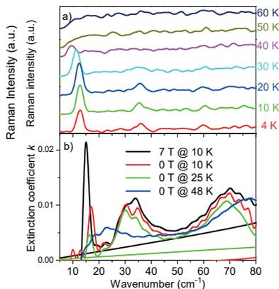
**Fig. 1. (a) Raman and (b) THz spectra of  $\text{Ni}_3\text{TeO}_6$  ceramics revealing two simultaneously detected spin excitations.**
