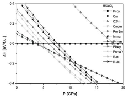
Fig. 1. Calculated enthalpy as a function of pressure for different phases of BiGaO<sub>3</sub>.
