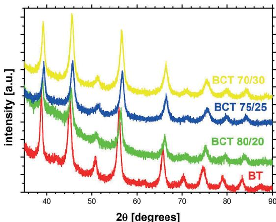
Fig. 1. XRD patterns of  $BaTiO_3$  and different  $Ba_{1-x}Ca_xTiO_3$  composition obtained after milling for 70 h.
