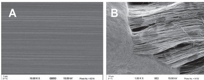
**Fig. 1.** Microstructure of Cu-Ag wire (a) and Nb multifilament nanowire with partially etched Cu matrix (b).
