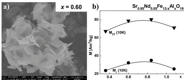
Fig. 1a SEM image of an agglomerate of  $\text{Sr}_{0.95}\text{Nd}_{0.05}\text{Fe}_{11.4}\text{Al}_{0.6}\text{O}_{19}$  crystallites; 1b remanence  $M_r$  and magnetization  $M$  measured in field of 2 T at 10 K.
