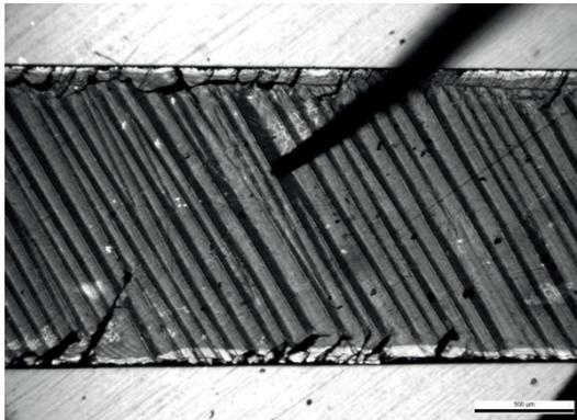
**Fig. 1. Pattern of CDWs in (111)<sub>c</sub> oriented BaTiO<sub>3</sub> single-crystal obtained by frustrative poling procedure across the phase transition from orthorhombic to tetragonal phase under UV light illumination.**
