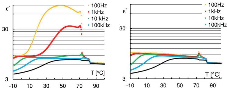
**Fig. 1.** Real part  $\epsilon'$  of electric permittivity for compound 1 versus temperature at five frequencies of measuring field (100 Hz, 1 kHz, 10 kHz, 100 kHz, 1 MHz). Left - no DC field, right - 10 V DC field.
