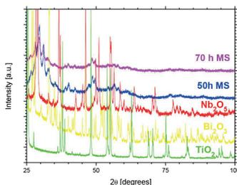
Fig. 1. XRD patterns of  $\text{Bi}_3\text{TiNbO}_9$  obtained after different milling periods.
