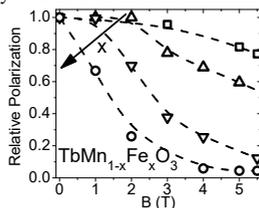
Fig. 1. Relative polarization of  $\text{TbMn}_{1-x}\text{Fe}_x\text{O}_3$ ,  $0 \leq x \leq 0.05$ , as a function of magnetic field.
