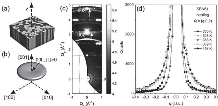
Fig. 1. Sketches (a) and (b) indicate a typical nanodomain structure of a uniaxial relaxor and the equi-intensity surface of the associated diffuse scattering. Example of this transverse diffuse scattering (c) in an intensity map of elastic scattering (indicated by arrows) at 380 K in SBN50 on IN20 and (d) in elastic scans at  $\mathbf{Q} = (q, 0, 2)$  in SBN61 single crystal on IN3 ILL, Grenoble.
