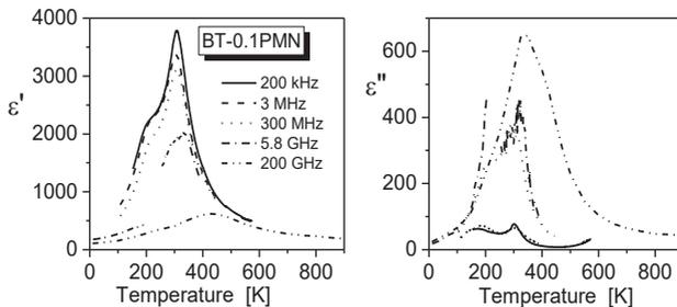
**Fig. 1. Temperature dependences of dielectric permittivity and loss of BT-0.1PMN at different frequencies.**
