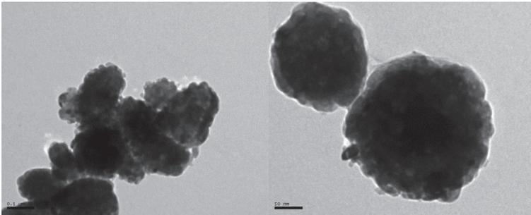
**Fig. 1. Transmission electron microscopy images of BaTiO<sub>3</sub>@NiO core-shell particles.**
