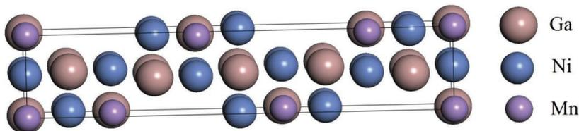
Fig. 1. The modulated 10M martensitic structure of Ni<sub>2</sub>MnGa alloy.
