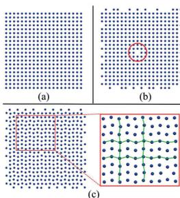
**Fig. 1. The atomic displacements in the two-dimensional square lattice with defects.**
