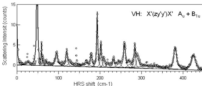
**Fig. 1.** Example of an HRS spectrum of  $PbZrO_3$  at 20 K (directions  $x'$  and  $y'$  are rotated by  $45^\circ$ ). All spectra were fitted by a sum of damped harmonic oscillators.
