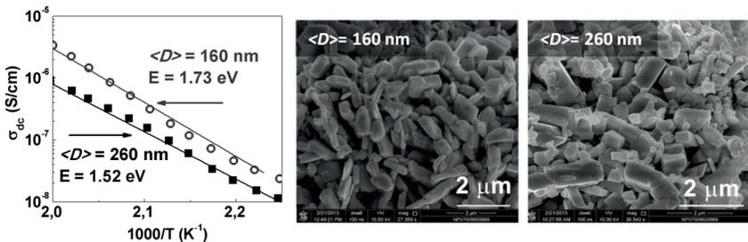
Fig. 1. High-temperature  $\sigma_{dc}$  conductivity versus reciprocal temperature (left), SEM images of BFO powder with crystallites of mean thickness  $\langle D \rangle = 160$  nm and  $\langle D \rangle = 260$  nm.
