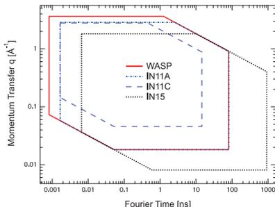
**Fig. 1. Dynamic window of the neutron spin-echo spectrometers at ILL.**
