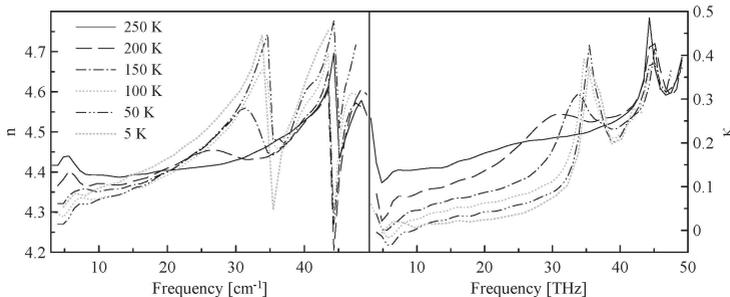
**Fig. 1.** THz spectra of the complex refractive index of  $(\text{Ba}_{0.2}\text{Sr}_{0.8})_3\text{Co}_2\text{Fe}_{24}\text{O}_{41}$  as a function of temperature.
