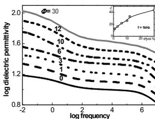
Fig. 1.  $\log \epsilon'$  versus  $\log f$  for BFO-PVDF nanocomposites of various volumetric fraction  $\Phi$  at room temperature.
