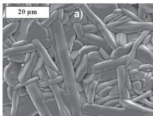
Fig. 2. Scanning electron microscope image of the fracture surface of  $\text{Bi}_3\text{TiNbO}_9$  obtained by conventional solid state sintering process.
