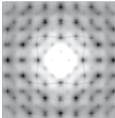
**Fig. 1. Diffuse scattering on the  $hk0.5$  reciprocal plane in the cubic phase of PZO comprising features related to correlated shifts of Pb atoms (intense blobs) as well as octahedra tilting (weak but sharp lines).**
