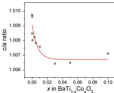
Fig. 1. Tetragonality of the BaTiO<sub>3</sub>:Co<sub>2</sub>O<sub>3</sub> structure as a function of nominal Co content in the BaTiO<sub>3</sub>:Co<sub>2</sub>O<sub>3</sub> samples.
