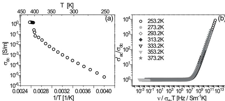
**Fig. 1. Arrhenius plot of AHS along a direction (a). Master curve of the real part of conductivity for AHS in low conducting phase (b).**
