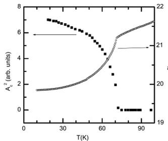
**Fig. 1. Temperature dependence of the dielectric constant (right) compared to the amplitude of the 100 antiferromagnetic peak of neutron diffraction (left).**
