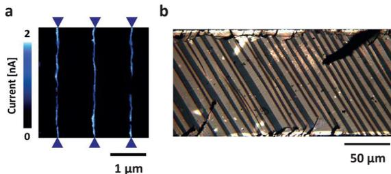
Fig. 1. (a) Conductive atomic force microscopy image of artificially created CDWs in 45 nm (001)<sub>c</sub> thick BiFeO<sub>3</sub> film on 5 nm SrRuO<sub>3</sub> electrode and DyScO<sub>3</sub> substrate [6], (b) Optical image of superbandgap illumination-created CDWs in (111)<sub>c</sub> BaTiO<sub>3</sub> single crystal.
