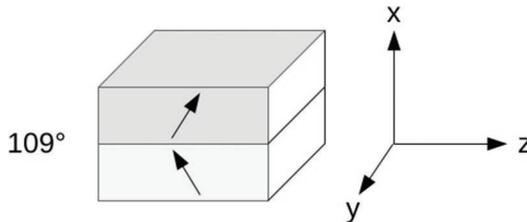
Fig. 1.  $109^\circ$ -DW structure.
