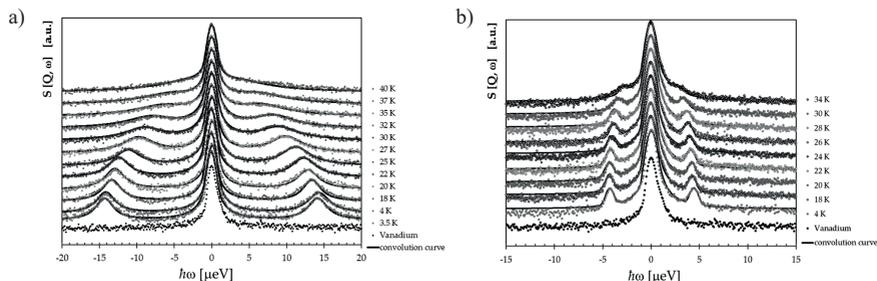
**Fig. 1. Tunneling results for (a) 2MP-CLA and (b) TMP-BRA complex at several temperatures in the energy range  $\pm 20$  and  $\pm 15$   $\mu\text{eV}$ , respectively [2].**
