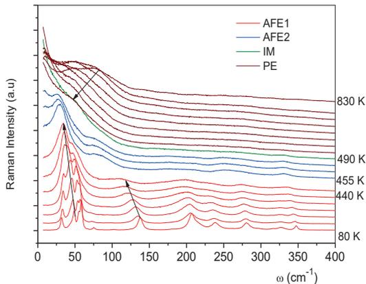
**Fig. 1. The evolution of the Raman spectra for  $\text{PbZr}_{0.72}\text{Sn}_{0.28}\text{O}_3$  in the A1, A2, IM and PE phases. All spectra are vertically displaced for clarity. Arrows indicate softening of certain modes.**
