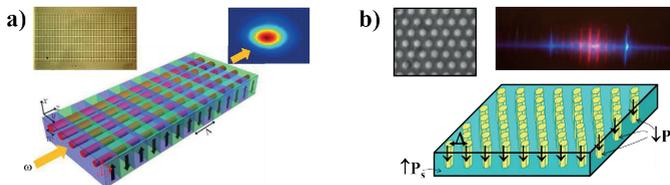
**Fig. 1. a) Periodically poled LiNbO<sub>3</sub> waveguide chips for all-optical signal processing, b) hexagonally poled ferroelectric domain lattices for multiple-beam optical frequency conversion.**
